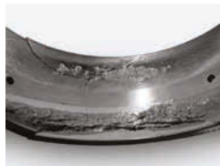
Pictured: outer ring flaking and crack damage.
